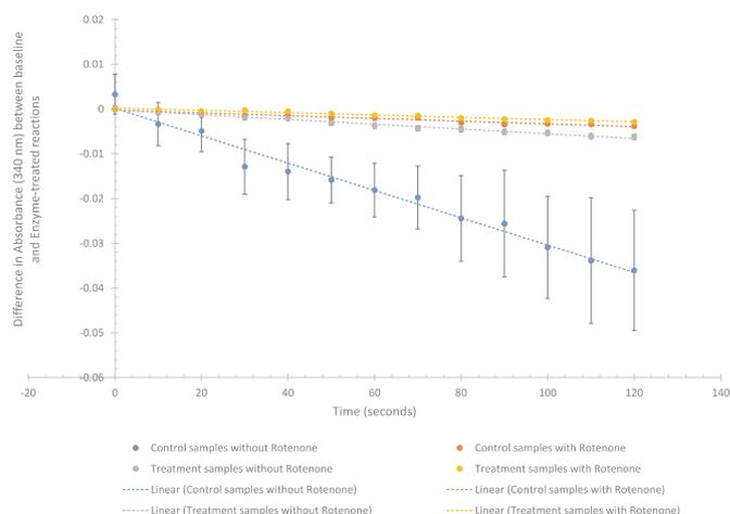
**Fig. 1.** Complex I activity. Oxidation of NADH demonstrated by a decrease in absorbance at 340 nm over a 2 min duration. Each data point represents data acquired from three different mitochondrial protein samples (biological replicates) obtained from Human colon carcinoma cells with wild type p53 (HCT-p53+/+) tested in triplicate (3 technical replicates). Errors bars represent standard error for  $n = 9$ .
